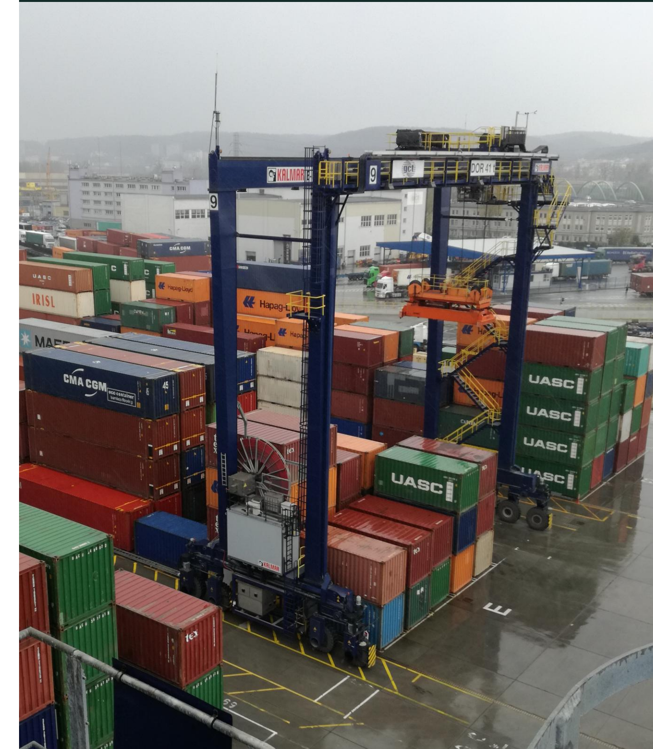
Suwnica typu - Rubber tired gantry (RTG)
