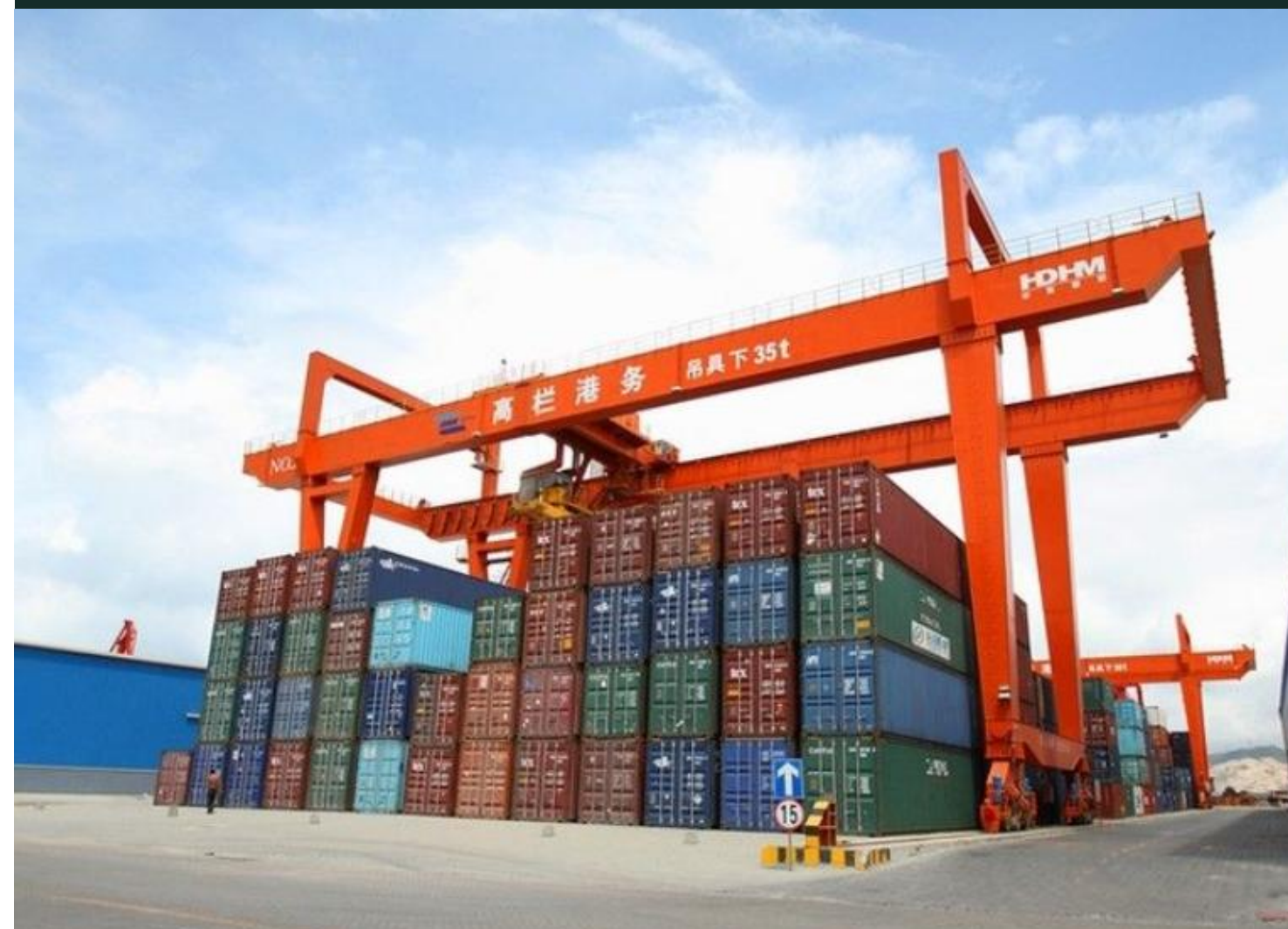
Suwnica typu - Rail mounted gantry (RMG)
