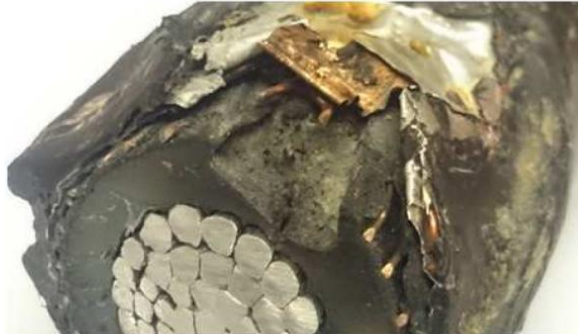
Fig. 1 Critical metallic screen connection points at termination, joint, and along cable with screen wires and metallic laminate
