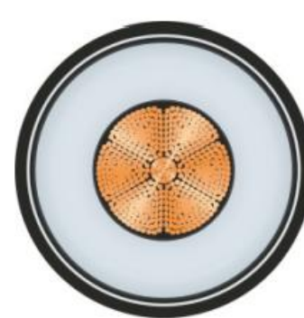
example 4: copper Milliken conductor with smooth welded aluminium sheath
